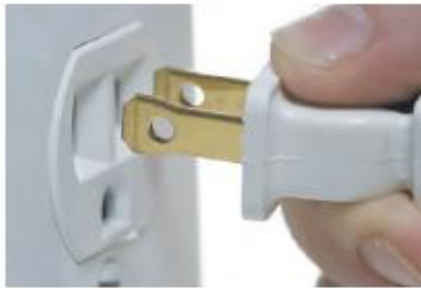
Figure 60 - This wall socket delivers a root-mean-square voltage of 120 V. Sixty times per second, the instantaneous voltage across its terminals varies from \sqrt{2}(120\text{ V}) = 170\text{ V} to -170\text{ V} and back again
