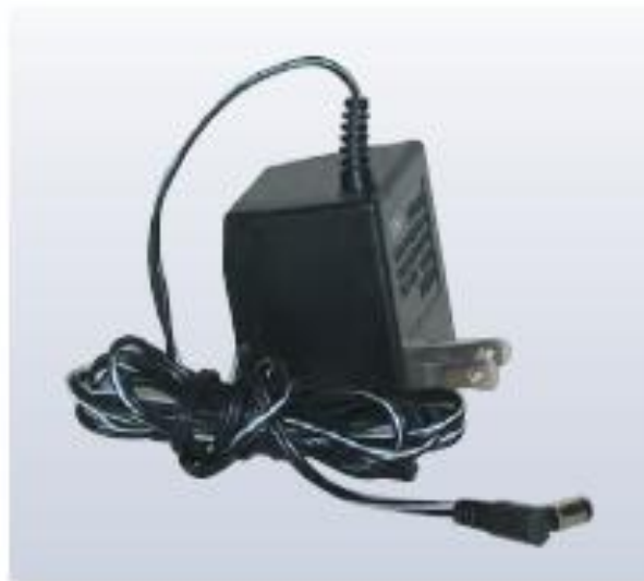
Figure 67 - An ac adapter like this one converts household ac into low-voltage dc for use in electronic devices. It contains a step-down transformer to lower the voltage and diodes to rectify the output current
