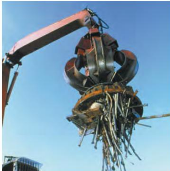
Figure 19 – This electromagnet contains a current-carrying coil with numerous turns of wire. The resulting magnetic field can pick up large quantities of steel bars and other iron-bearing items
